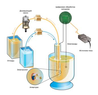
This results in a small change in the voltage in the amplifier, which converts variance in current into a pulse. The height of the pulse is proportional to the particle size and sufficient to give a precise measurement of the particle.
