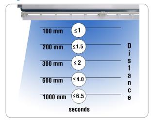
µWire AeroBar Model 5710 (500 mm length) with 50 mm Air Jet Spacing. Measured using Simco-Ion CPM Model 280A w/HEPA flow (60 fpm or 0.3m/sec) & CDA flow at 50 lpm.
