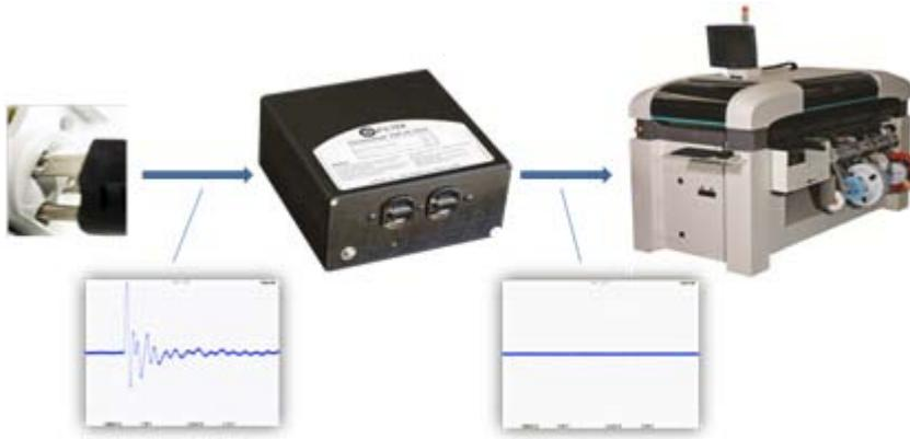
**Figure 10 Connection of Power Line EMI Filter**
