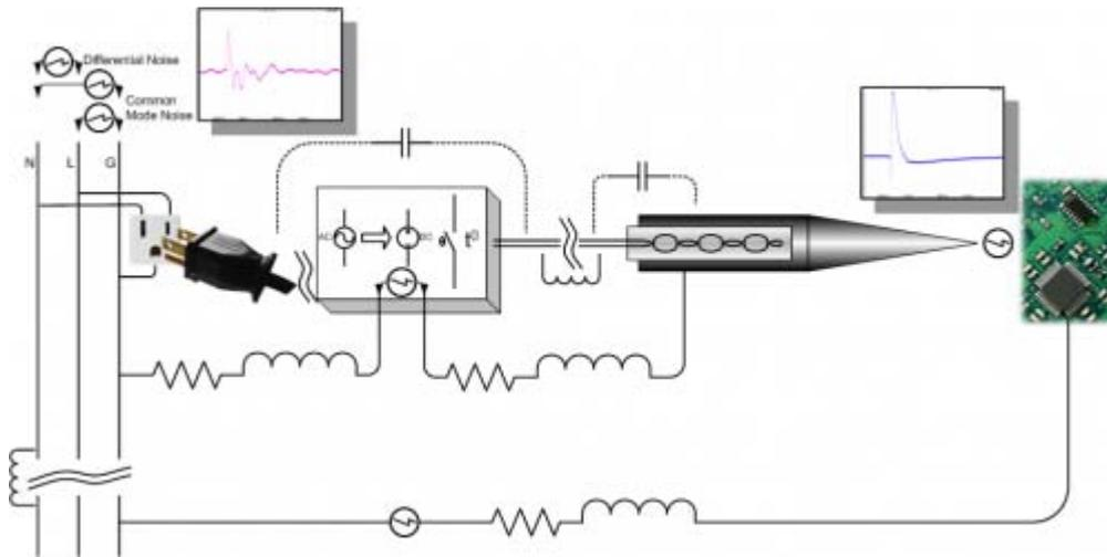
**Figure 5 Noise Propagation in the Soldering Iron**
