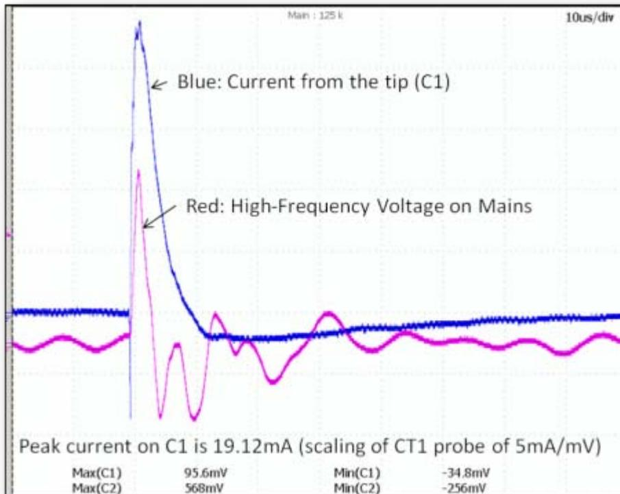
**Figure 4 Transient on power line from periodic signal and resulting current from the tip**
