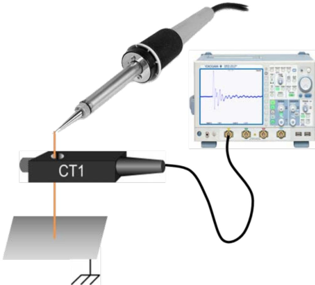
**Figure 3 Test Setup for Measuring EOS Exposure**
