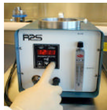
9) When the test period is complete, stop the sample cycle, or the sample cycle will self terminate at the end of the pre-set test period interval.
