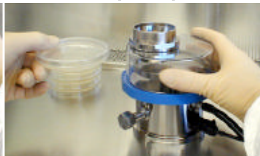
12) Replace the dome assembly to keep the sample chamber contaminant free until the next test plate is employed.
