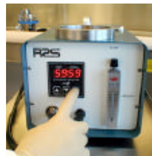
6) Set the desired test period interval (from 1" to 59'59") and start the sample cycle.
