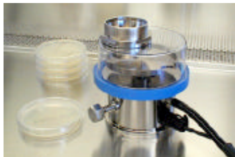
1) Sanitize the R2S (sampler) and place at the desired test location. Ensure that the vacuum & power cable connections are secure.
