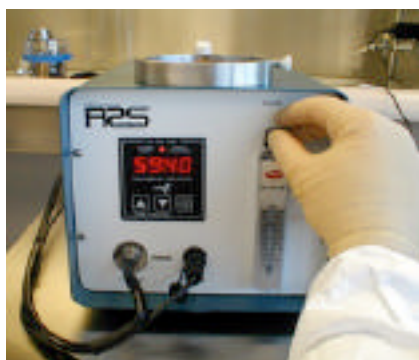
7) Ensure that the sample flow rate is set to the specified set point for 60 SCFH (or 1 CFM) on the flowmeter.
