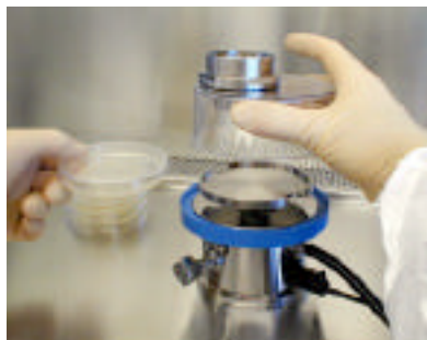
2) Remove the dome assembly, retaining it over the sampler to minimize the risk of incidental contamination.
